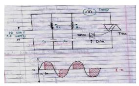
In this method, the limitation of thyristor operated dimmer is overcome. The triac is nothing but two SCR connected back to back and gate terminal is common. It will conduct +ve or –ve half cycles.
