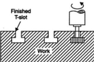
Figure:T-Slot milling operation.
