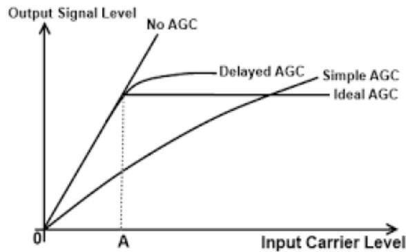
Figure (c): AGC Characteristics for Various Techniques
