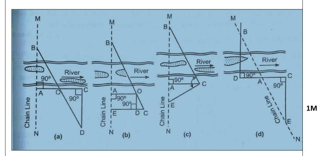
Fig-a) A & B are two points on opposite banks of river as shown in fig 1. obstructed length is AB on the chain line MN , Set AC perpendicular to AB & bisect at O . Errect perpendicular at C & mark a point D in a line with BO, measure the length CD, from principle of similar triangles ABO & CDO, AB = CD
