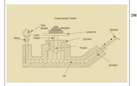
• The dead weight tester apparatus consists of a chamber which is filled with oil and a piston – cylinder. The top portion of the piston is attached with a platform to carry weights. A plunger with a handle has been provided to vary the pressure of oil in the chamber. The pressure gauge to be tested is fitted at an appropriate plate.
