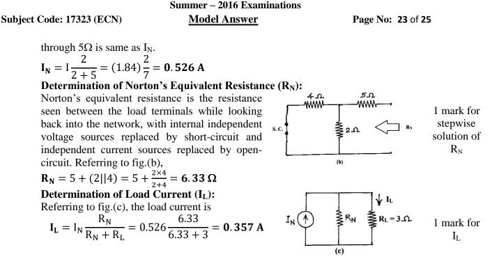
6 d) State Norton's theorem and write its procedural steps to find current in a branch (Assume a simple circuit).
