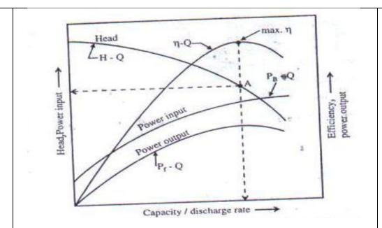
The H-Q curve shows the relationship between head and capacity rate .it is clear from the curve that the head decreases continuously as the discharge rate is increased. The optimum conditions for operation are those at which the ordinate through the point of maximum efficiency cuts the head curve. The point A is called as duty point.
