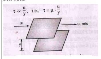
Consider two layer of fluid 'y' cm apart as shown in fig. Let the area of each of these layer be A cm<sup>2</sup>. Assume that top layer is moving parallel to the bottom layer at a velocity u cm/s relative to the bottom layer. To maintain this motion i.e. the velocity 'u' and to overcome the fluid friction between these layers, for any actual fluid, a force of 'F' dyne is required.
