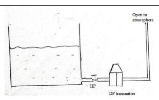
A differential pressure (DP) transmitter mounted near the bottom of the tank measures the pressure of the liquid inside it. A valve at the bottom side of the vessel is connected to the high pressure (HP) side of the DP and the low pressure side is vented to atmosphere.
