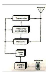
**Transmitter:** It is low power FM unit operating in the frequency range of 825 to 845MHz. There are 666, 30 KHz transmit channel. The carrier is furnished by a frequency synthesizer is a phase modulated by voice signal.
