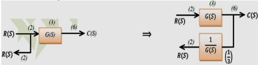
iv) Shifting a take off point before a block: To shift take off point before a block, we shall add a block with transfer function  $G$  in series with signal which is taking off from that take off point.
