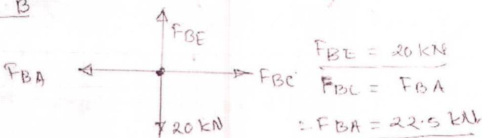
$$\frac{F_{BE} = 20 \text{ kN}}{F_{BC} = F_{BA}} \quad (1\text{M})$$
