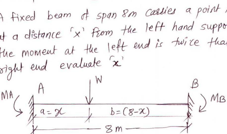
$MA = 2MB \quad \text{--- (I)}$ <p>To find fixed end moments.</p> $MA = -\frac{Wab^2}{L^2} = -\frac{W(x)(8-x)^2}{8^2}$ $MB = -\frac{Wa^2b}{L^2} = -\frac{W(x^2)(8-x)}{8^2}$ <p>Putting values of MA &amp; MB in equation I</p> $\therefore -\frac{W(x)(8-x)^2}{8^2} = 2 \left[ -\frac{W(x^2)(8-x)}{8^2} \right]$ | <p>Any<br/>TWO<br/>for<br/>TWO<br/>marks.</p> <p>1 Mark</p> <p><math>\frac{1}{2}</math> Mark</p> <p><math>\frac{1}{2}</math> Mark</p> <p>1 Mark</p> |
