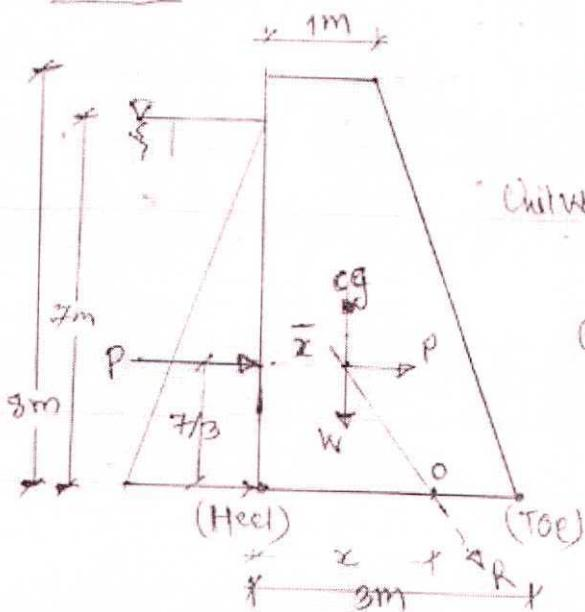
Unit wt. of water =  $10 \text{ kN/m}^3$ Unit wt. of masonry =  $22 \text{ kN/m}^3$
