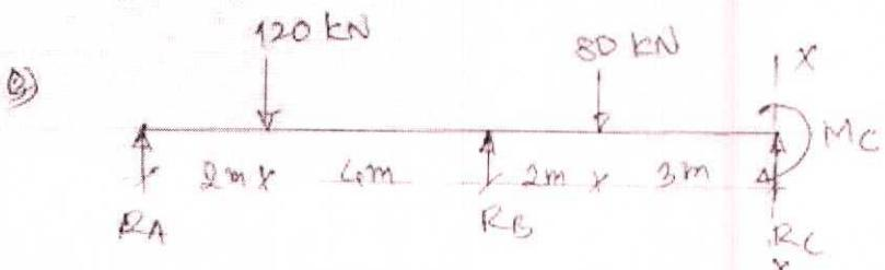
$$\text{BM at section x-x} - (RA \times 11) + (RB \times 5) - (120 \times 9) - (80 \times 3) \\ = -59.58$$
