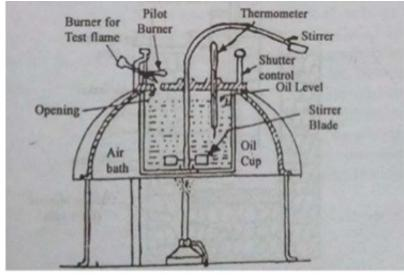
Clean the cup & fill it with given sample of oil up to the filling mark. Cover the cup with lid. Thermometer is inserted and it should not be touch the metallic cup. Heat the oil by means of electric heater or burner so that the 3
