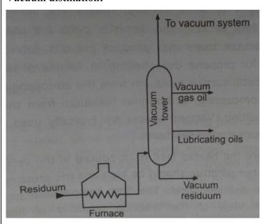
Heavier fractions from atmospheric distillation unit that cannot be distilled without cracking under its pressure & temperatureconditions are vacuum distilled. Vacuum distillation is simply distillation of petroleum fractions at
