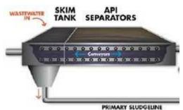
API Separators: API or American Petroleum Institute Separators are normally the first and most important step in a refineries wastewater treatment. It uses the differences in oil and water's specific gravity to filter out the majority of
