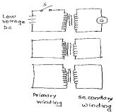
i) This test is carried out on 3-ph transformer to identify primary & secondary winding belonging to the same phase.
