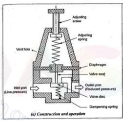
The diaphragm type pressure reducing valve consists of a diaphragm, made up of synthetic rubber, allows the proper movement for opening and closing of valve, without mechanical friction. The topside of diaphragm is in contact with lower spring rest where as the bottom side of diaphragm is contact with valve pin. This pin moves the valve from its seat.
