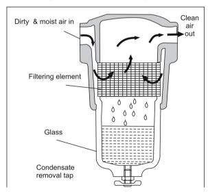
The choice of type of filters depends upon the quality of air required, the normal air conditions, and accessibility to filter for repair or replacement of filtering element. Figure 19.1 shows a typical filter (mechanical type and using impregnated felt as the filter element).
