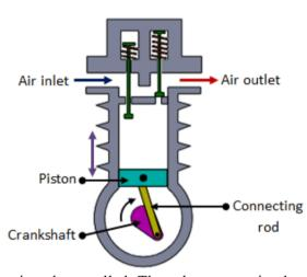
Ans: Piston compressors are commonly used in pneumatic systems. The simplest form is single cylinder compressor shown in figure. It produces one pulse of air per piston stroke. As the piston moves down during the inlet stroke the inlet valve opens and air is drawn into the cylinder. As the piston moves up the inlet valve closes and the exhaust valve opens which allows
