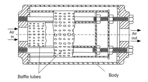
Muffler is a device which is used in the pneumatic system to reduce the noise created by exhausting air. It does exactly what a silencer does in an automobile.Mufflers are attached to the exhaust port of air valves, cylinders or motors. Several designs have been developed, some of them patented by various manufacturers but with the central core of dissipating the exhaust energy.
