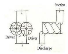
A screw compressor is one of the rotary type air compressors, which is being widely used in modern plants, with sophisticated controls. A screw compressor as the name implies, consists of two rotating screws. Both screws are synchronized either by external timing gears or by one screw driving the other by contact. As the screw rotates air is drawn into the housing, trapped between the screws and carried along to the discharge port, where it is delivered in a constant pulse free stream. Working :
