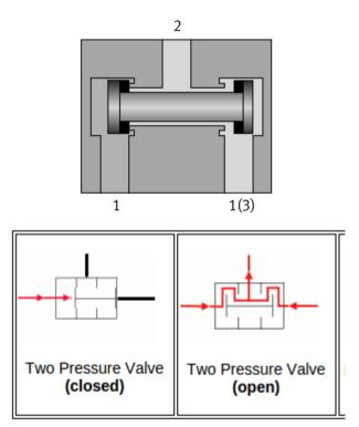
These valve types are commonly associated but not limited to safety circuits, for example a two push button operation system whereby an operator is required to use both hands to activate two push buttons, this would ensure the operators hands are out of reach of any hazardous operations.
