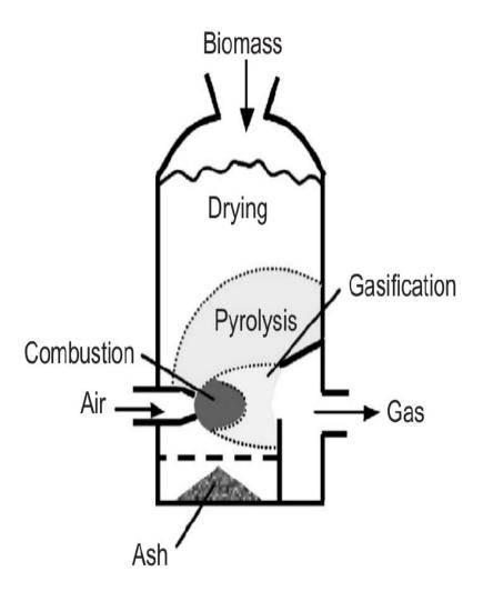
\* Cross draft gasification is one of the simplest types of gasification; the reactor for this gasification is much like the updraft gasifier in that the fuel will enter from the top and the thermochemical reaction will occur progressively as this fuel descends into the reactor.
