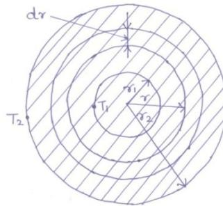
**(a) Heat flow through thick walled cylinder**
