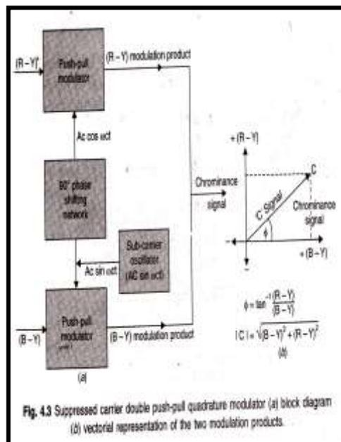
The push pull modulator not only suppressed the carrier but also eliminates the higher harmonics and enables easy addition of the quadrature outputs to form chrominance signal.
