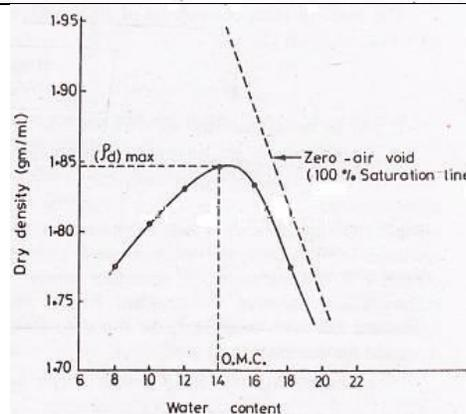
Figure : Standard proctor compaction test
