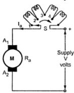
iii) For same torque if field coil is arranged in series or parallel MMF of coil changes, hence flux produced also changes and speed can be controlled. Some fixed speeds can only be obtained. In parallel grouping higher speeds can be obtained.
