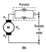
Any one method of armature control diagram 1 mark and explanation 1 mark
