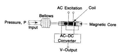
It consists of a primary winding (or coil) and two secondary windings (or coils). The windings are arranged concentrically next to each other. They are wound over a hollow bobbin which is usually of a non-magnetic and insulating material. A ferromagnetic core (armature) is attached to the transducer sensing, shaft (such as bellows). The core is generally made of a high permeability ferromagnetic alloy and has the shape of a rod or cylinder.
