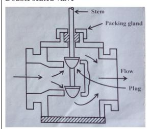
In double seated valve, there are two plugs. The flow moves upward in one
