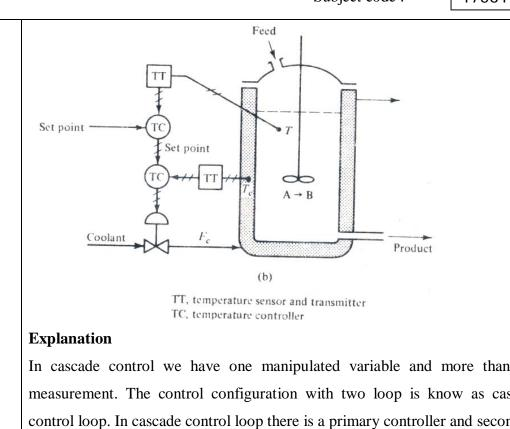
In cascade control we have one manipulated variable and more than one measurement. The control configuration with two loop is know as cascade control loop. In cascade control loop there is a primary controller and secondary controller. The output of primary controller is given as a set point to secondary controller. Disturbance arising the secondary loop are corrected by the secondary loop before the affect the value of the primary controlled output.
