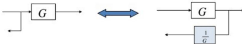
ix) Moving summing point after a block: To shift summing point after a block, another block having transfer function  $G$  is added before the summing point.
