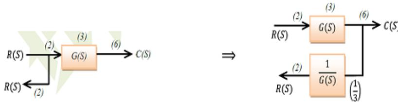
iv) Shifting a take off point before a block: To shift take off point before a block, we shall add a block with transfer function G in series with signal having taking off from the take off point
