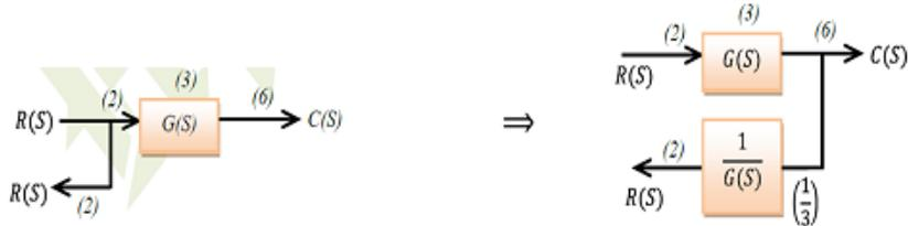
iv) Shifting a take off point before a block: To shift take off point before a block, we shall add a block with transfer function  $G$  in series with signal having taking off from the take off point
