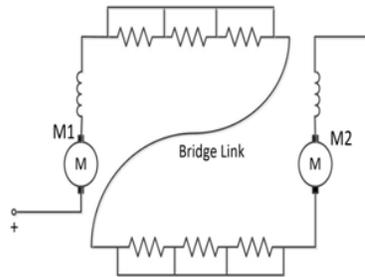
Step2: Bridge link is so rotated that two motors are put in series without starting resistance. Which are un-shorted at the same time.
