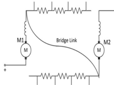
Step 3: The portions of external resistance are connected in each motor circuit as shown in fig
