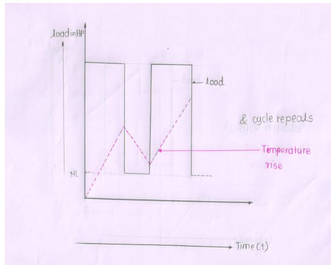
**Explanation** :-In this case motor is operated continuously for long time and interval between two load is not OFF- load but motor runs at no load for short time. So temperature of drive continuously increases.
