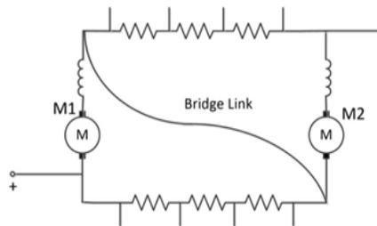
Step4: In this last step bridge link is removed as shown in fig. This is nothing but parallel first step.
