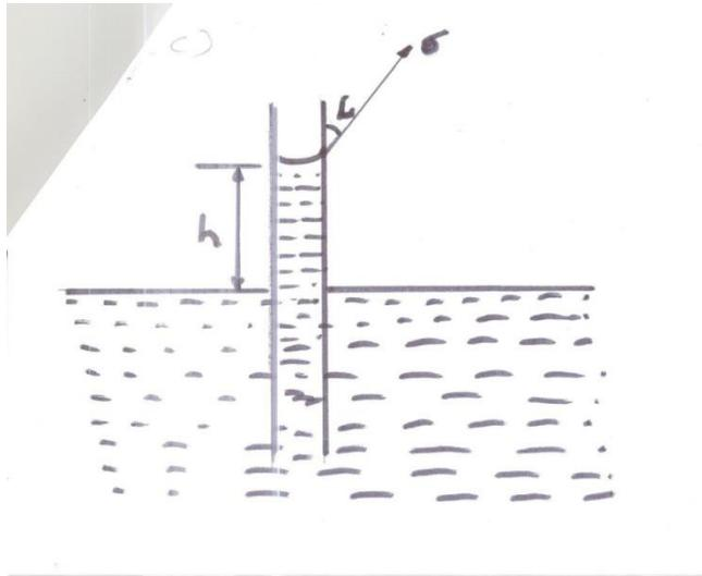
Weight of the water column in the tube above the water surface acting downwards-
