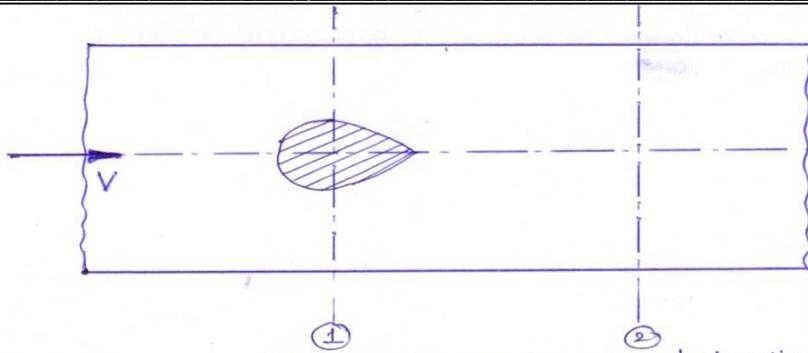
Fig - Head Loss due to obstruction
