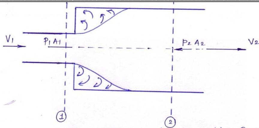
Fig-Head Loss due to sudden Expansion
