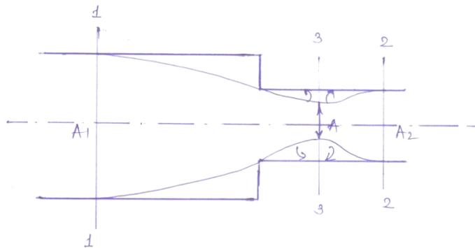
Fig-Loss of head due to sudden contraction.
