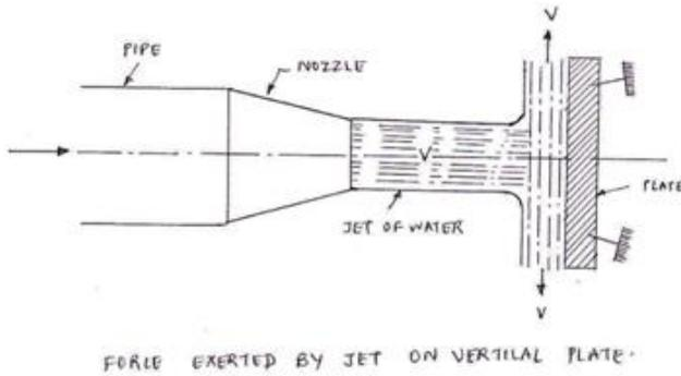
Consider a jet of water coming out from the nozzle, strikes a flat vertical plane as shown in fig.
