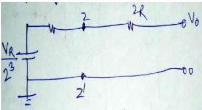
Similarly for digital input 010 and 100 the equivalent voltages are  $V_R/2^2$
