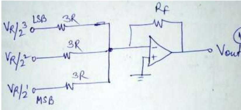
The analog output voltage for a given digital input is given by
