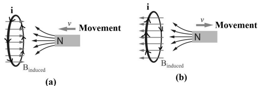
If the direction of movement of magnet is reversed to take it away from the loop, the loop experiences decrease in the flux. The emf now acts to oppose the decay in the flux. So the emf circulates loop current in such direction that the flux produced by loop current lies in the same direction as the flux of magnet. For this the emf circulates current in clockwise direction as shown in the figure (b). Thus the emf always acts to oppose the cause of its production.
