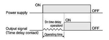
The on-delay operation is an operation to give output when preset time expires after a predetermined input is given to the power supply circuit or input circuit.
