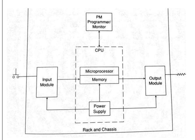
The main parts of a PLC are,
