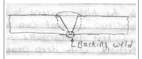
One or two layer of weld metal is applied on the underside of the seam to support weld metal that will be deposited from the opposite side.
