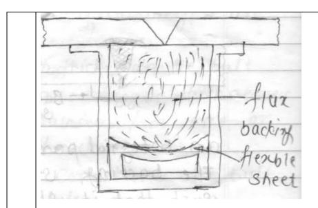
Moderate flux pressure is developed on the back side of the weld.
