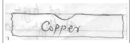
Bar grooved or ungrooved straight or circular is used to support molten weld pool. Such a bar does not fuse and became a permanent part of weld .Copper chills molten metal rapidly.
