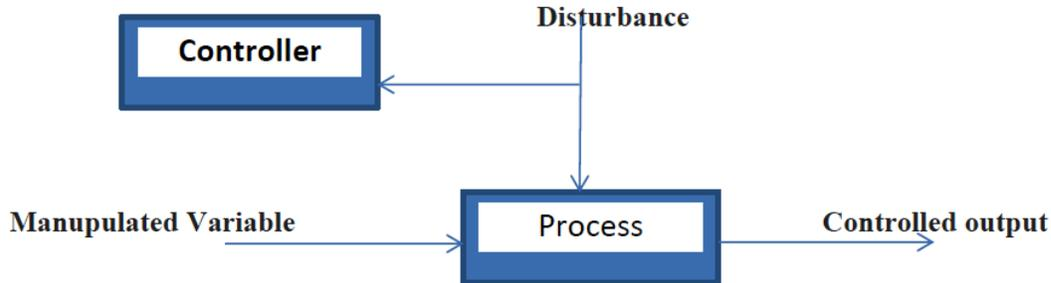
**Fig. Feed Forward control system**
