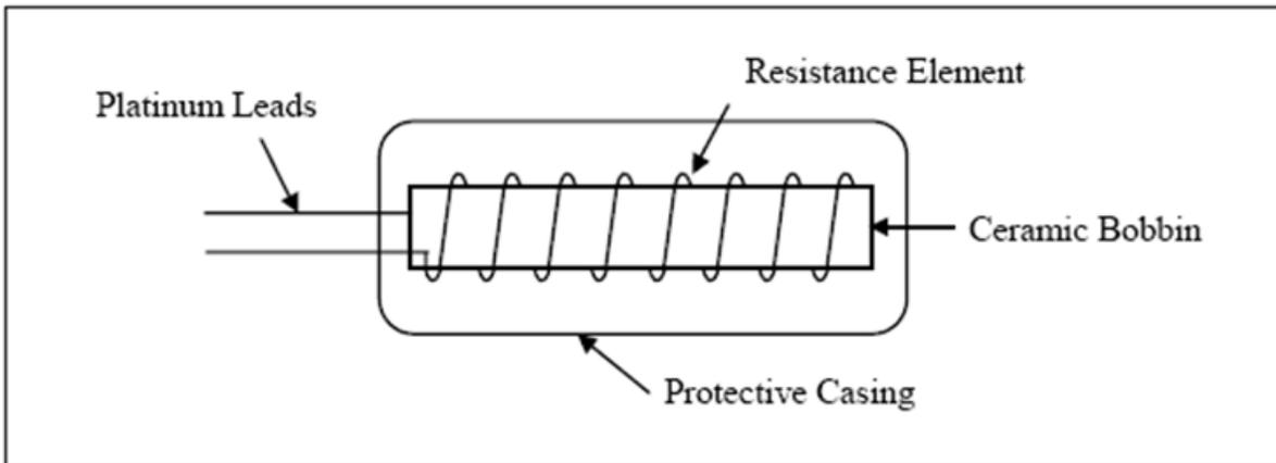
The certain metals changes with temperature change. Resistance thermometer utilizes this property of the material. With the increase in temperature the electrical resistance of the certain material increases in direct proportion to rise the temperature. Therefore if electrical resistance of wire of known and calibrated material is measured the temperature of the wire can be determined. Platinum, copper and nickel are generally used in resistance thermometers
