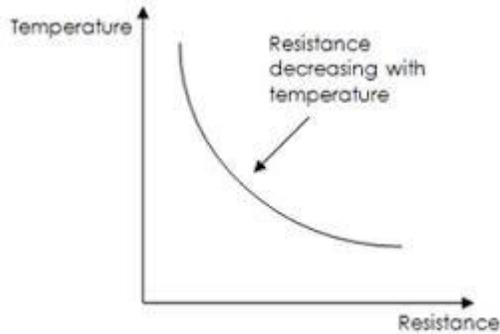
These are made up of ceramic like semi conducting materials like copper oxide ,manganese oxide ,nickel oxide, cobalt oxide, Lithium oxide and titanium oxide.
