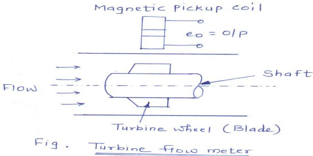
The turbine flow meter works on the principle of turbine. if the losses are kept minimum the turbine speed varies linearly with flow rate i.e flow rate can be measured by measuring the speed of the turbine. When the blade passes by pick up coil, it interrupt magnetic field and produces a pulse. The rate of pulse gives flow rate and total number of pulses gives a measure of the total flow.
