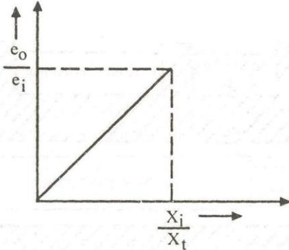
Under ideal circumstances, the output voltage varies linearly with displacement as shown in figure.
