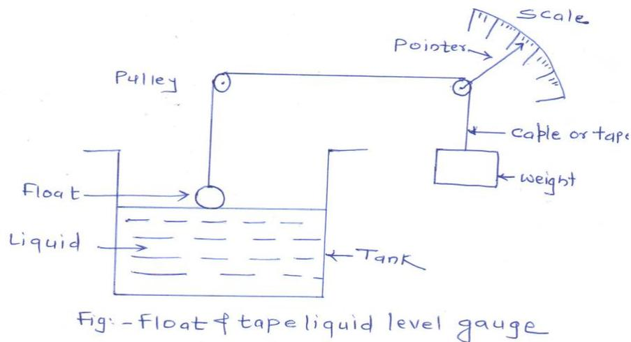
In this, a freely floating body (float) is used for continuous liquid level measurement. The float is attached to the cable /tape which passes over the pulley and then at another end of tape, the weight is applied for counter-balancing of force.
