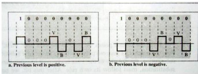
**HDB3 Code:** It is a modification of AMI code & overcomes the problem of long string of binary 0s. If there are more than three consecutive zeros, a violation pulse (V) is substituted for the fourth zero. The violation pulse has the same polarity as the last pulse & it is easily identified at the receiver end.
