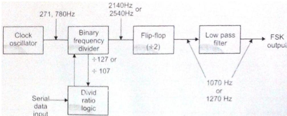
Note that binary 1 corresponds to frequency 1270 Hz and binary 0 to frequency 1070 Hz
