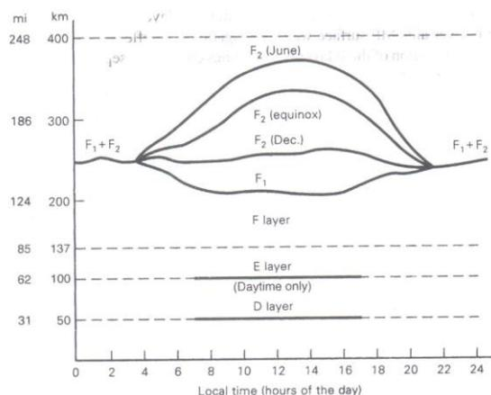
The ionosphere is the upper portion of the atmosphere. It absorbs large quantities of radiant energy from the sun, get heated and ionized. There are variations in the physical properties of
