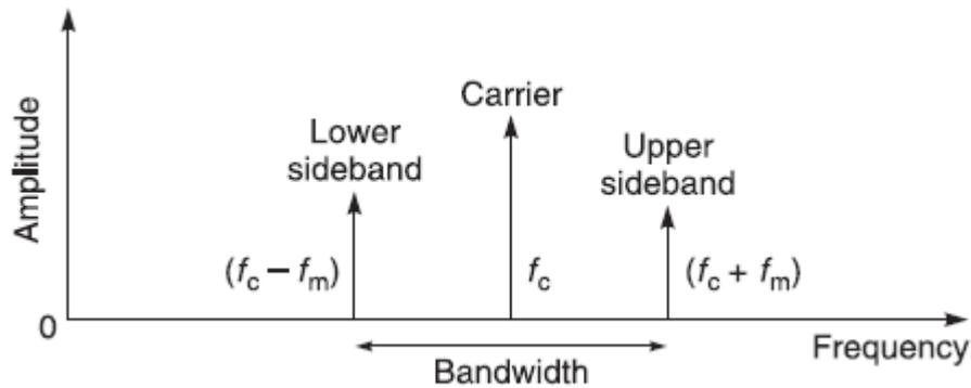
Bandwidth= $2f_m$  where  $f_m$  is frequency of modulating signal
