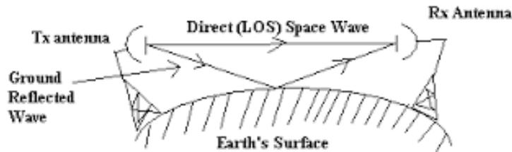
Figure :- Space Wave Propagation
