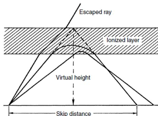
When the wave is refracted by the ionosphere it is bent down gradually rather than sharply. Below the ionized layer, the incident and refracted rays follow path that are
