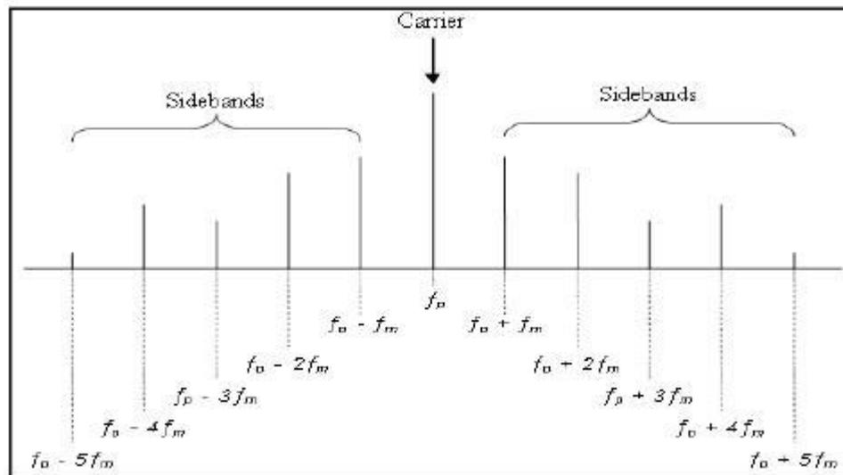
Figure 3. An FM signal's frequency spectrum
