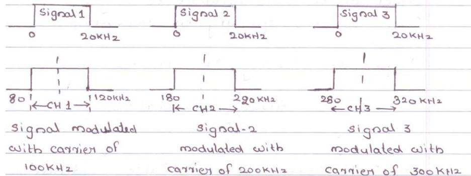
3. **To increase the range of communication:** the frequency of the baseband signal is low. Therefore it cannot travel a long distance, when they are transmitted. They get heavily attenuated. The attenuation of signal reduces with increase in frequency of the transmitted signals and they travel long distance. The modulation process increases the frequency of the signal to be transmitted. Hence modulation increases the range of communication.
