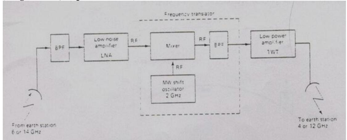
A typical satellite transponder consists of :
