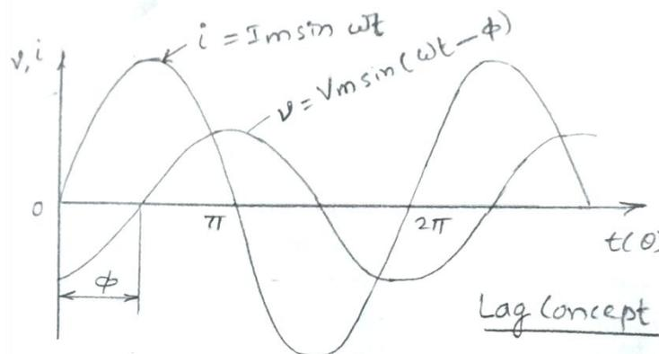
**Lagging Phasor Representation:** Voltage (V) lagging current (I) by angle  $\Phi$
