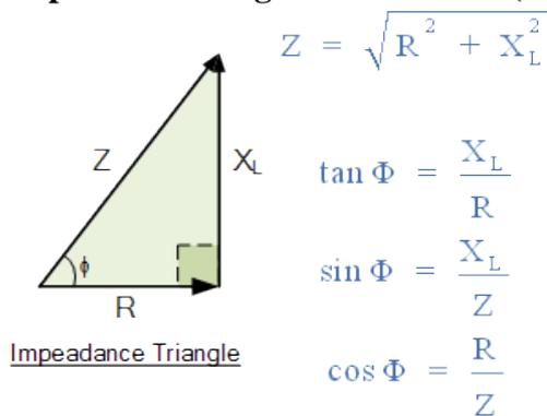
e) A choke coil is connected across 230 V, 50 Hz supply. The power consumed by the coil is 960 W and current is 8amp. Calculate circuit constants (R and L).
