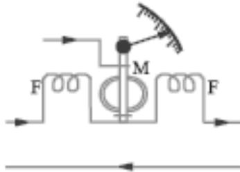
Where F = Fixed Coil; M – Moving Coil
