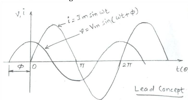
**Leading Phasor Representaion:** Voltage (V) leading current (I) by angle  $\Phi$
