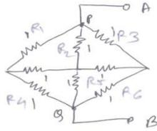
As shown in fig, one end of resistors  $R_1, R_2$  &  $R_3$  are connected to Node P. And  $R_4, R_5$  &  $R_6$  are connected to Q. Hence star connection is formed.
