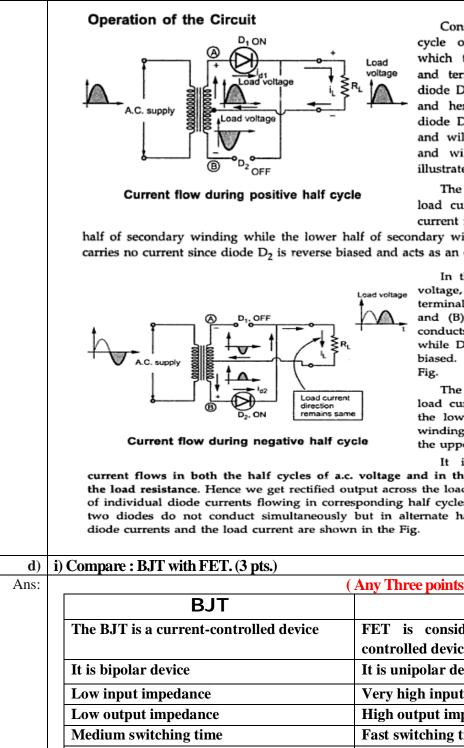
Consider the positive half cycle of ac input voltage in which terminal (A) is positive and terminal (B) negative. The diode D1 will be forward biased and hence will conduct; while diode D2 will be reverse biased and will act as an open circuit and will not conduct. This is illustrated in the Fig.
