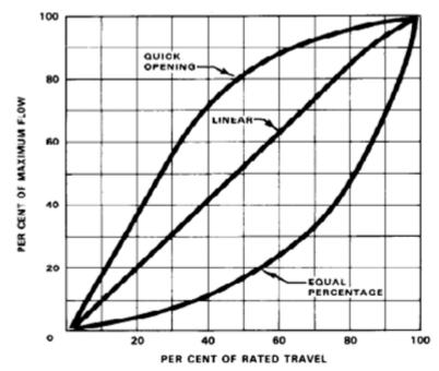
**Inherent flow characteristics** are plotted when constant pressure drop is maintained across the valve. There are two different inherent flow characteristics- linear and equal percent.
