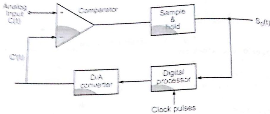
In this, the step size of the DAC is automatically varied depending on the amplitude characteristics of the analog input signal. When the output of the transmitter is a string of consecutive 1's or 0's, this indicates that the slope of analog signal either in +ve or -ve direction. The DAC has lost track of exactly where the analog samples are and the possibility of slope overload occurring is high. In ADM, the value of delta changes in accordance with the slope of the sampled analog input.
