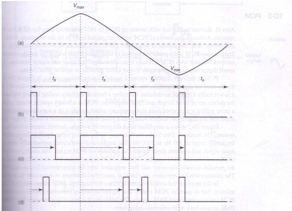
b) Define sampling theorem and draw waveform for natural sampling.
