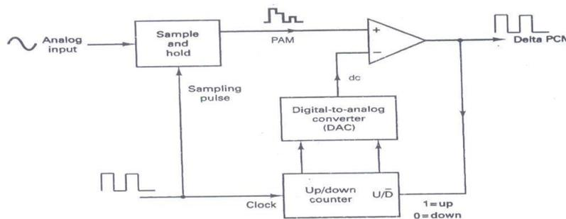
FIGURE 10-20 Delta modulation transmitter
