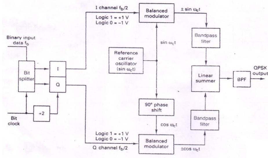
1. Two bits (a, dibit) are clocked into the bit splitter.
