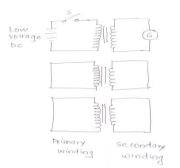
i) This test is carried out on 3-ph transformer to 1 m identify primary & secondary winding belonging to fi the same phase.
