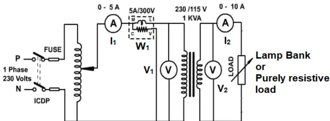
**Direct loading test on Single-phase Transformer**
