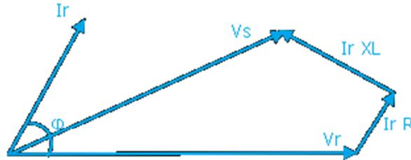
Capacitive load, receiving end voltage  $V_r$  is more than sending end voltage  $V_s$
