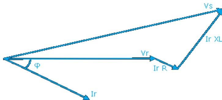
**∴ Inductive load, receiving end voltage  $V_r$  is less than sending end voltage  $V_s$**
