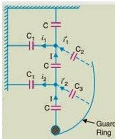
Guard ring is a metal ring electrically connected to conductor and surrounding the bottom insulator.
