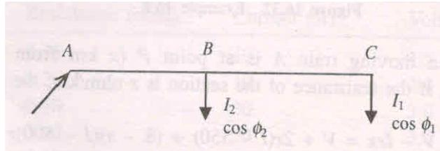
Consider a distributor with two loads  $I_1$  and  $I_2$  at power factors  $\cos \phi_1$  and  $\cos \phi_2$  respectively, as shown in above figure . Taking voltage at point C ( $V_C$ ) as reference, the phasor diagram is shown in below figure
