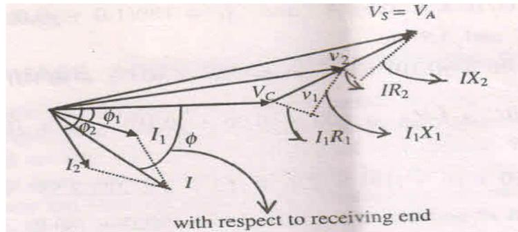
If the resistance of section  $BC$  is  $R_1 + jX_1$  and of section  $AB$  is  $(R_2 + jX_2)$ , the voltage drop in section  $BC$  will be  $\bar{I}_1(R_1 + jX_1)$  and in section  $AB$  it will be  $(\bar{I}_1 + \bar{I}_2)(R_2 + jX_2)$ ,
