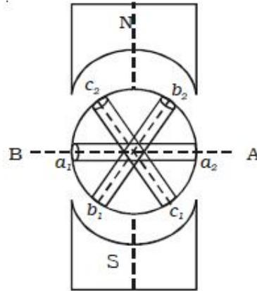
Fig: a Section of 3 phase ac generator
