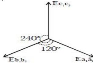
Fig: c Angular displacement between the armature
