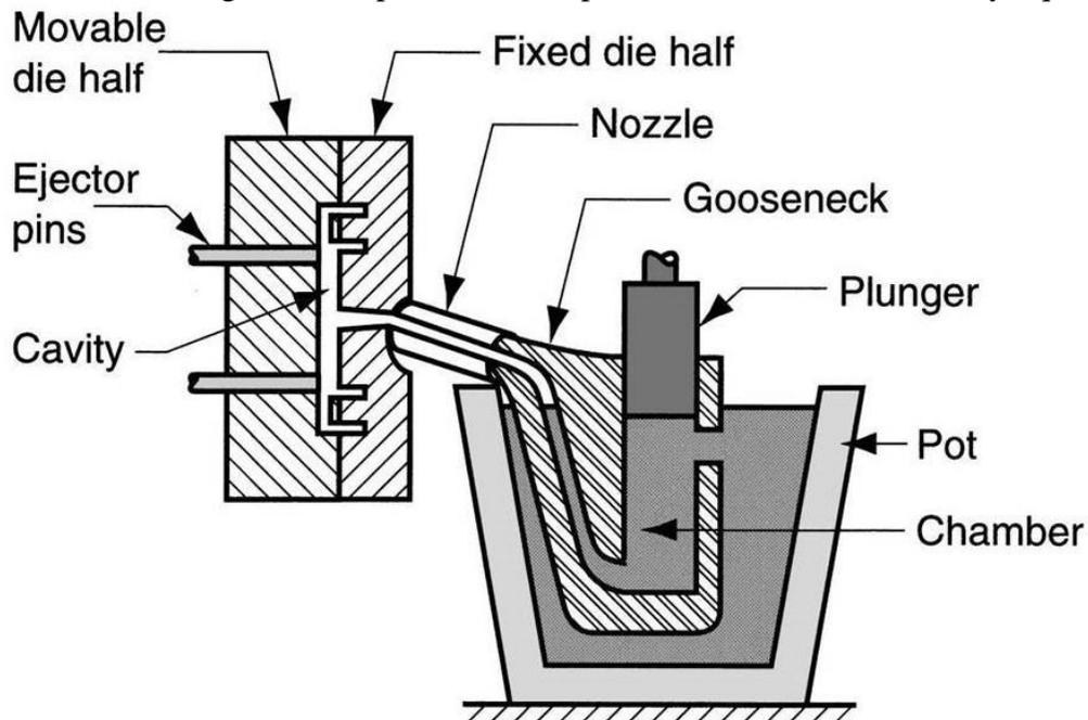
**Figure: Hot chamber die casting**
