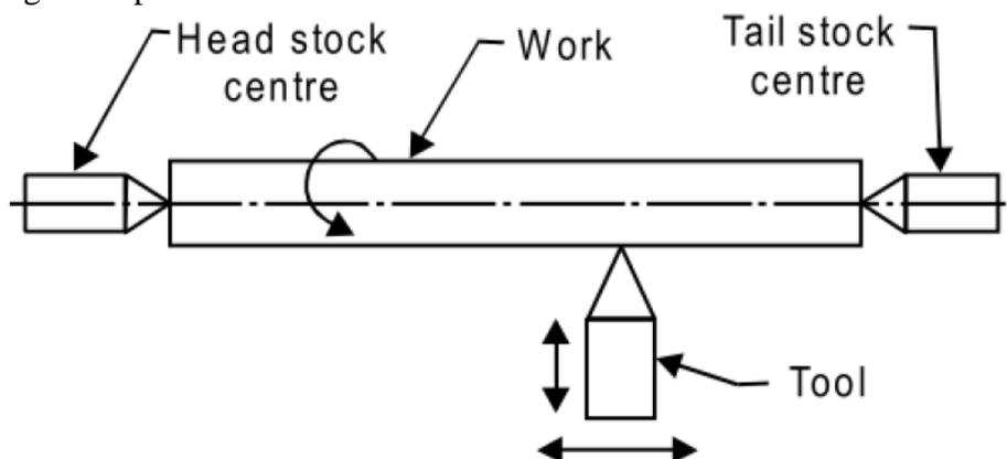
The working principle of a lathe is shown in Fig.
