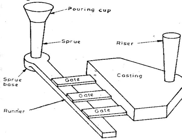
Figure: Gating system in casting.
