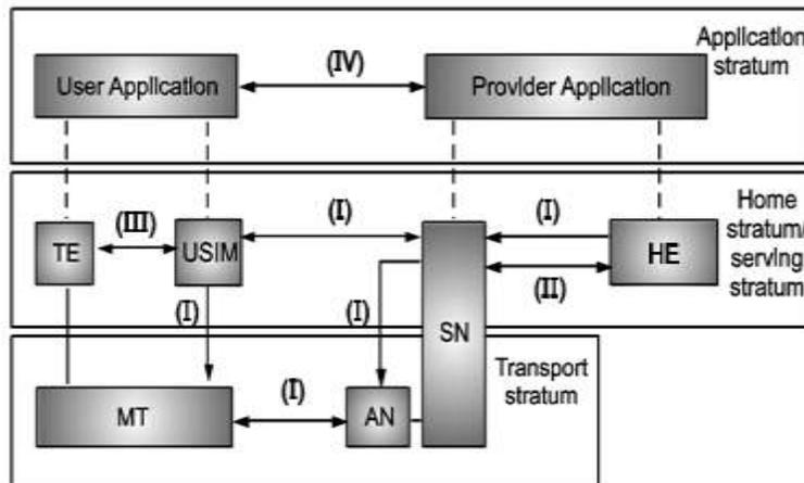
**Fig Overview of the 3G security architecture**
