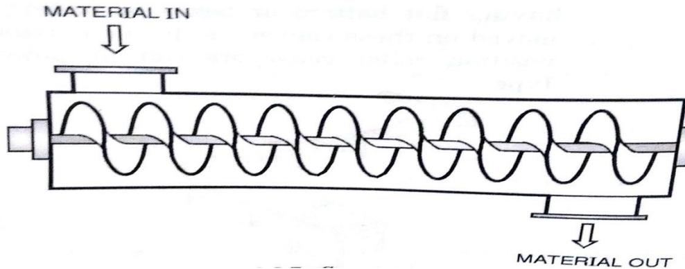
**Fig: Screw Conveyor.**
