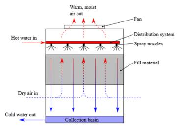
**Effectiveness.** This is the ratio between the range and the ideal range (in percentage), i.e. difference between cooling water inlet temperature and ambient wet bulb temperature, or in other words it is = Range / (Range + Approach). The higher this ratio, the higher the cooling tower effectiveness. CT Effectiveness (%) =  $100 \times (CW \text{ temp} - CW \text{ out temp}) / (CW \text{ in temp} - WB \text{ temp})$
