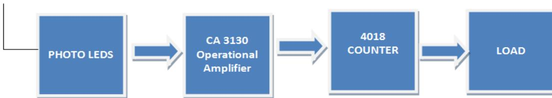
**Block Diagram of Infrared Remote Control Switch**
