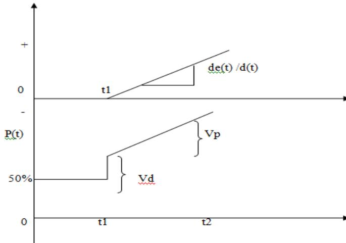
The ramp function of error occurs at  $t=t_1$ . The derivative mode causes a step  $V_d$  at  $t_1$  & proportional mode causes a rise of  $V_p$  equal to  $V_d$  at  $t_2$ .
