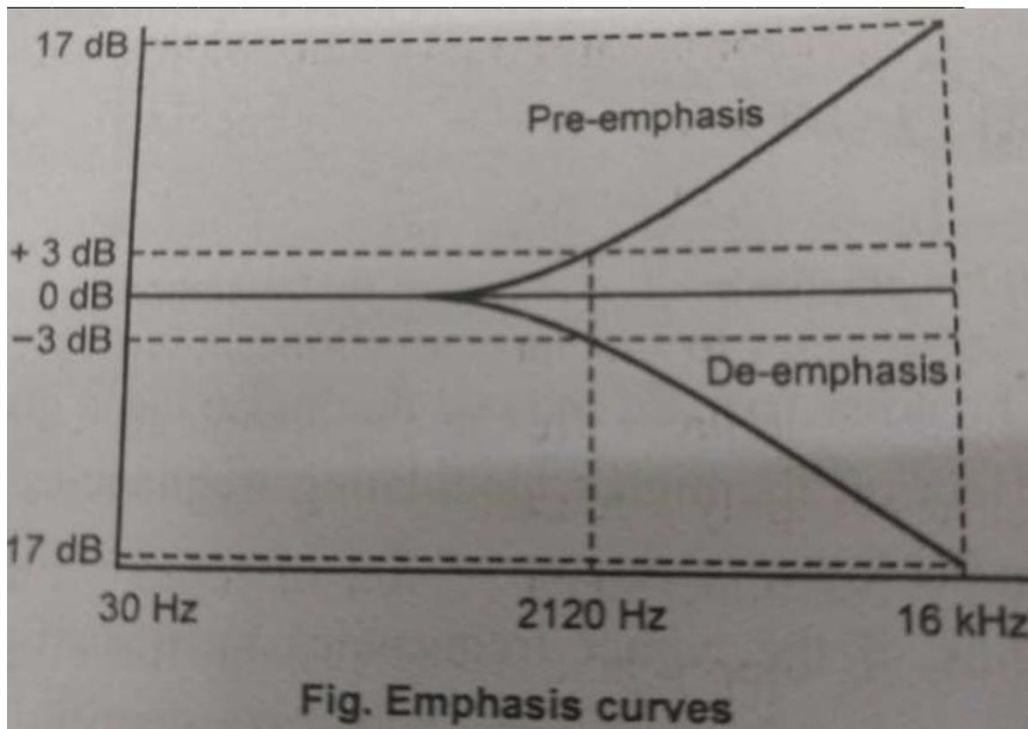
In FM, noise has greater effect on higher modulating frequencies than the lower one. Therefore the higher modulating frequencies have to be boosted artificially at the transmitter before modulation and corresponding cut off at the receiver after demodulation.
