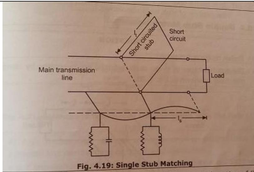
1. The most important feature of single stub matching is that the stub should be located as near to the load as possible.
