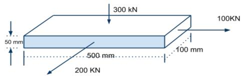
What is the change in the volume of the bar? take modulus of elasticity of 200GPa and poisson's ratio as 0.25.
