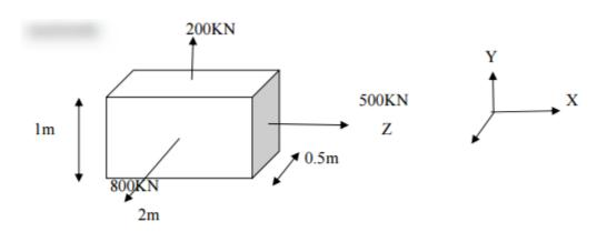
Find linear strains in x, y and z directions of the rectangular block loaded as shown in the figure. Hence using the linear strains values, find the total strain in z direction. Take E= 200GPa, and Poisson's ratio= 0.25
