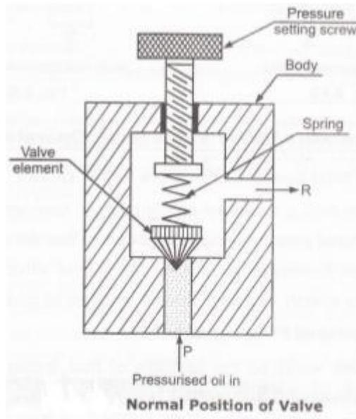
Fig. Pressure relief valve
