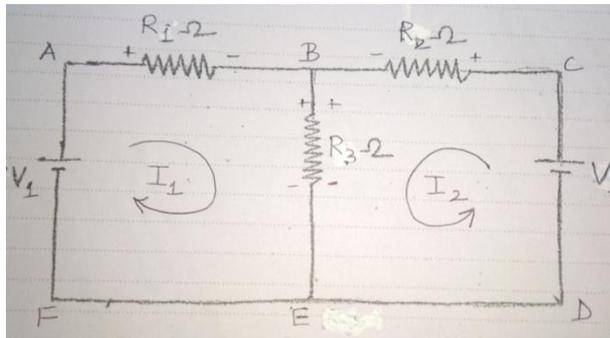
Applying KVL to Loop ABEFA,  $V_1 - I_1 R_1 - (I_1 + I_2) R_3 = 0$
