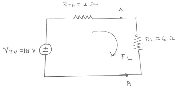
$$I_L = \frac{V_{TH}}{R_{TH} + R_L} = \frac{18}{2 + 6} = 2.25 \text{ A.}$$
