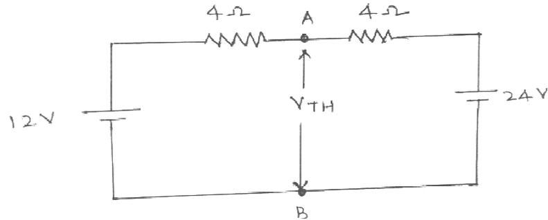
$$V_{TH} = 24 \text{ V} + \text{voltage across } 4 \Omega$$
