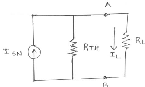
Determine the load current ( $I_L$ ) using equation,
