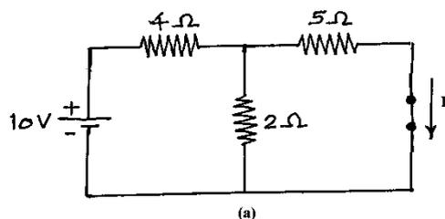
**Step IV:** Determination of Norton's Equivalent Resistance ( $R_N$ ):
