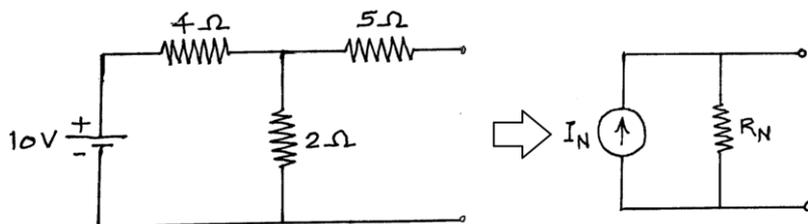
**Step III:** Determine of Norton's Equivalent Current Source ( $I_N$ ):
