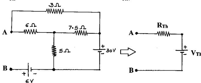
**Determination of Thevenin's Equivalent Voltage Source ( $V_{Th}$ ):**
